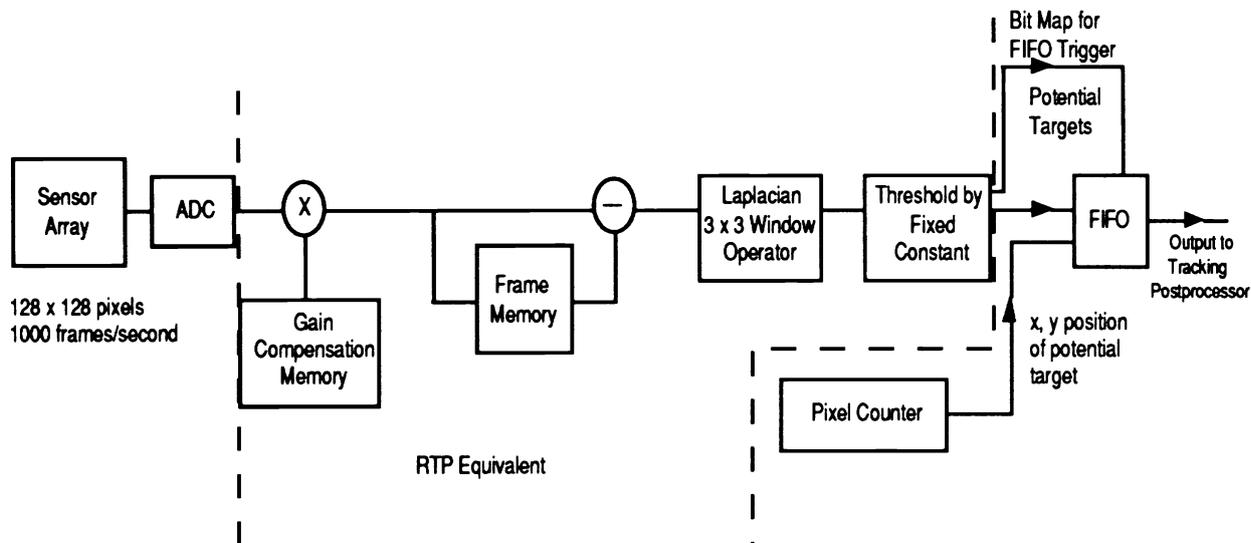
Fig. 1. Implementation of RTP functions with digital processing - data flow/functional diagram.
