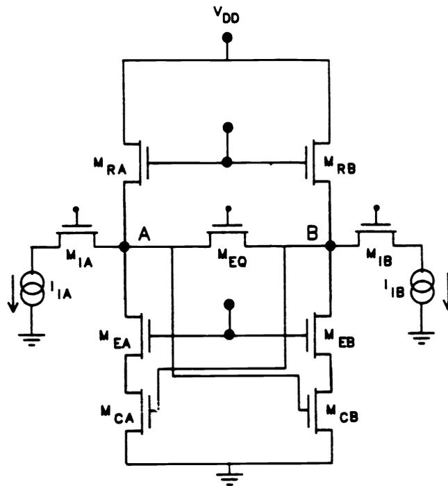
Fig. 4. The comparator schematic as simulated.
