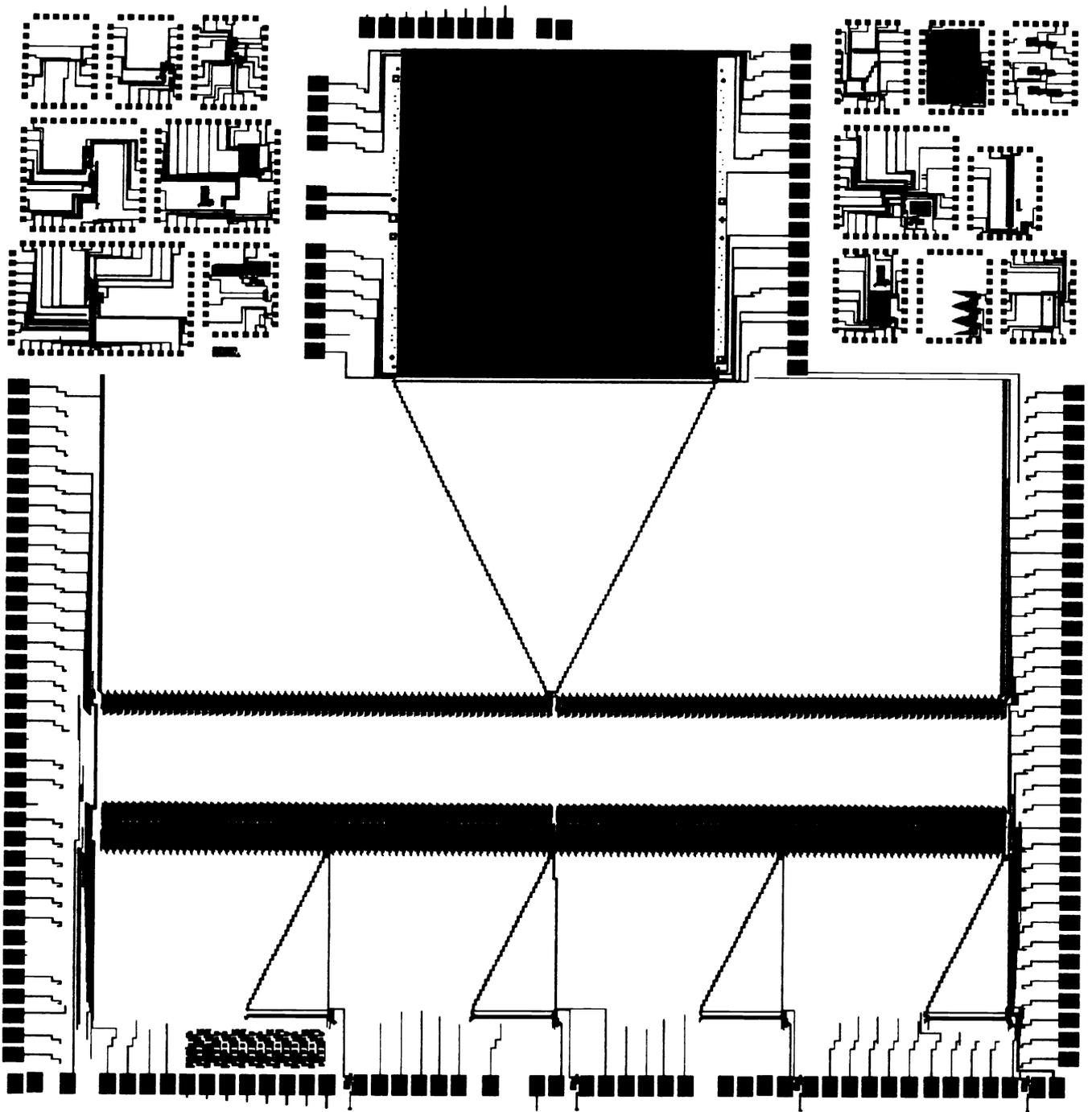
Fig. 3. First metal chip plot showing location of 128x128 multiplexer and pads.
