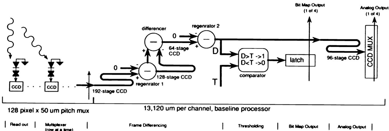
Fig. 2. Block diagram of processor channel.
