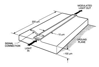
Fig. 2 Sketch of the MQW modulator.
