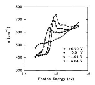
Fig. 5 Absorption spectrum of the test MQW waveguide modulator at various applied voltages.
