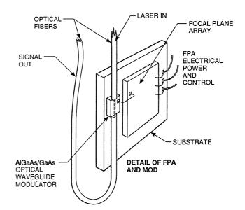
Fig. 1 Sketch illustrating the readout link concept.
