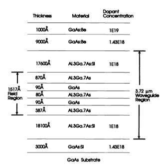
Fig. 4 Layer structure of the test MQW waveguide modulator.
