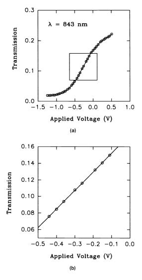
**Fig. 7** Modulation transfer function, optical transmission versus applied voltage at  $\lambda = 843$  nm: (a) complete curve and (b) magnified plot of the boxed region in (a).
