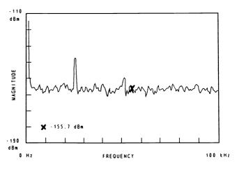
Fig. 8 Measured noise versus frequency spectrum of link output from 0 to 100 kHz.
