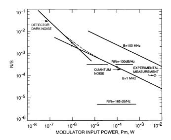
Fig. 3 Link relative noise versus modulator input power.
