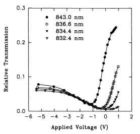
Fig. 6 Relative transmission versus applied voltage of the test MQW modulator at various wavelengths.
