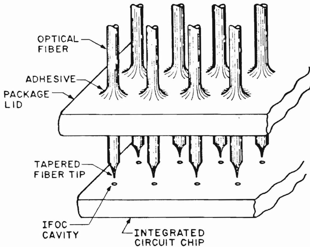
Figure 5. "Spaghetti extruder" package lid concept. Might be useful for aligning and vertically stabilizing arrays of optical fiber interconnections.
