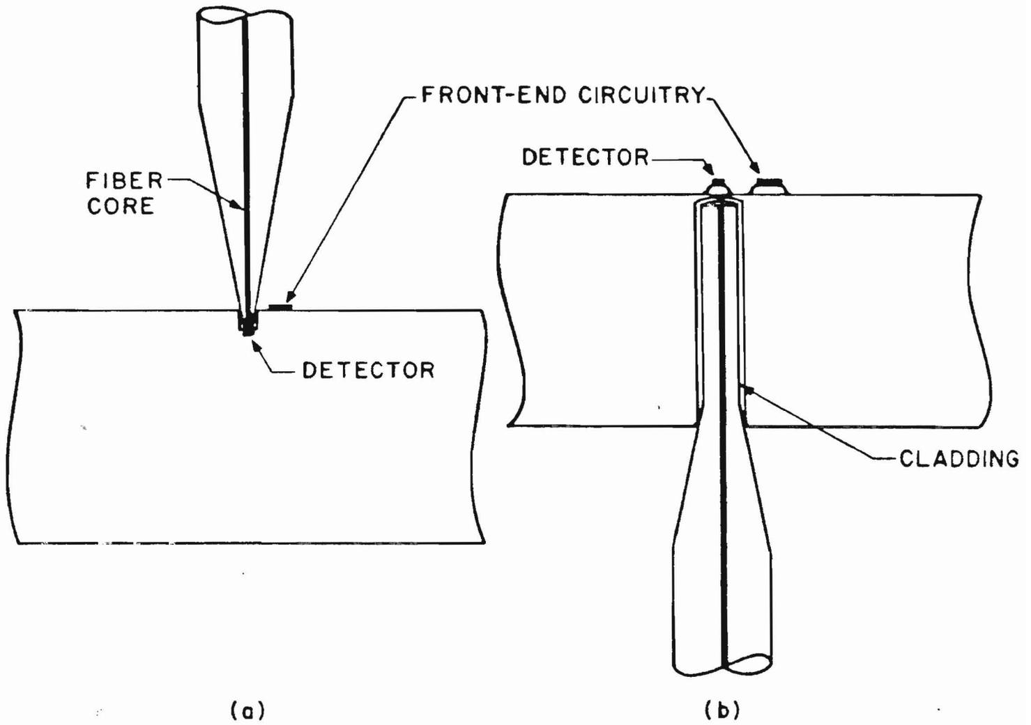
Figure 1. Illustration of (a) front-side and (b) backside integrated fiber-optic coupler concepts.
