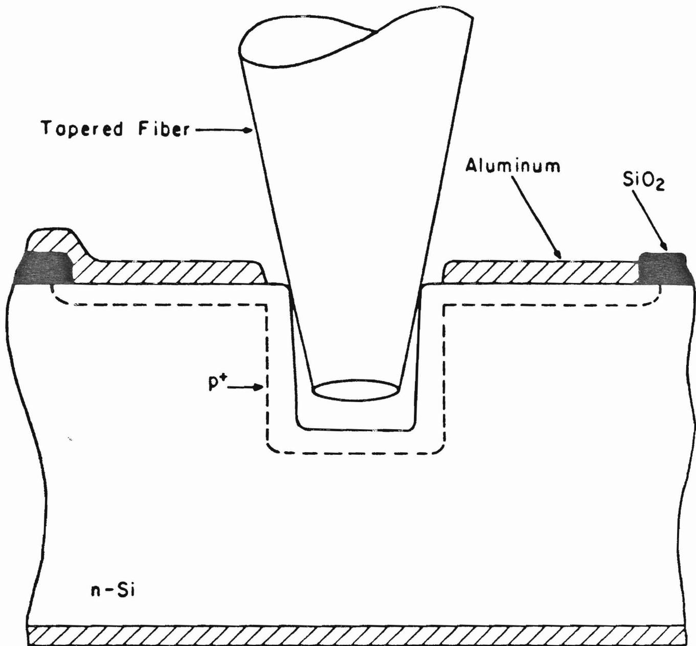
Figure 2. Cross-section of prototype front-side silicon detector IFOC structure.
