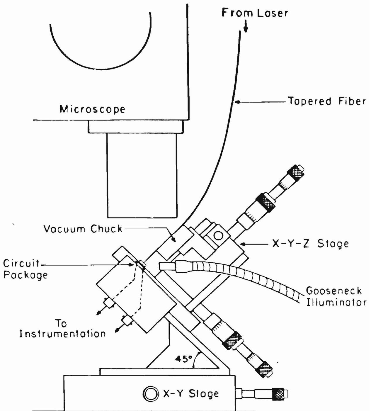
Figure 3. Schematic drawing of the work station used to insert optical fibers into the IFOC cavity.
