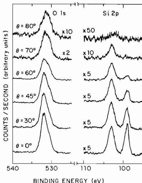
FIG. 2. Angle-dependent XPS spectra of ion-beam grown oxide. The Si 2p peak with lower binding energy ( $\sim 99$  eV), which disappears near grazing angle, corresponds to the substrate. The peak with higher binding energy ( $\sim 103$  eV) corresponds to the oxide.
