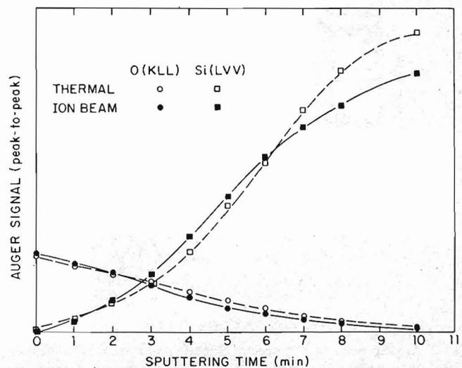
FIG. 1. AES depth profiles of thermally grown and ion-beam grown oxides.
