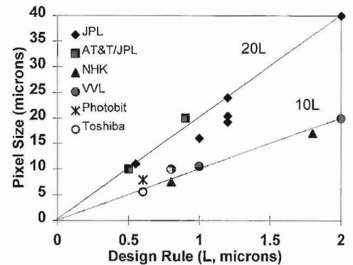
Fig. 9. Scaling trend in pixel size versus design rule. It is expected that pixel pitch must be between 5 and 10 μm to be competitive.
