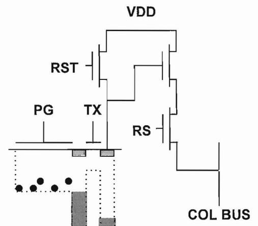
Fig. 5. Photogate-type APS pixel schematic and potential wells. Transfer of charge and correlated double sampling permits low-noise operation.
