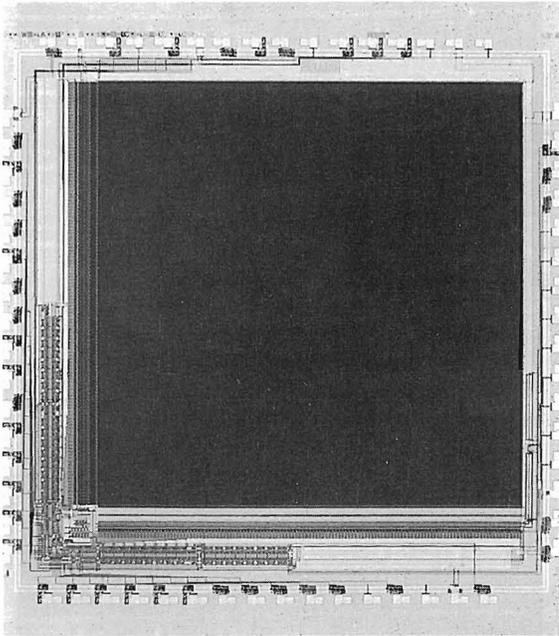
Fig. 6. A JPL  $256 \times 256$  element PG-APS with on-chip timing and control circuits (left-hand side) and analog signal chain including fixed pattern noise suppression (bottom).
