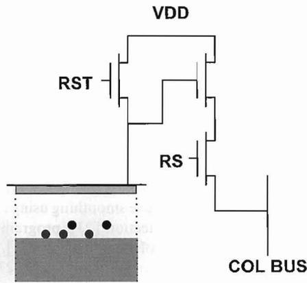
Fig. 3. A photodiode-type active pixel sensor (APS). The voltage on the photodiode is buffered by a source follower to the column bus, selected by RS-row select. The photodiode is reset by transistor RST.
