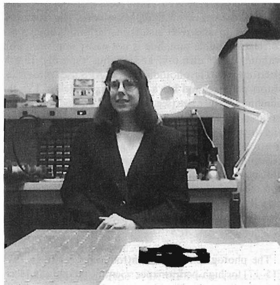
Fig. 7. Unprocessed image taken from a Photobit  $256 \times 256$  element sensor with on-chip ADC operating at 30 fps. Note no blooming from light and lack of other artifacts.
