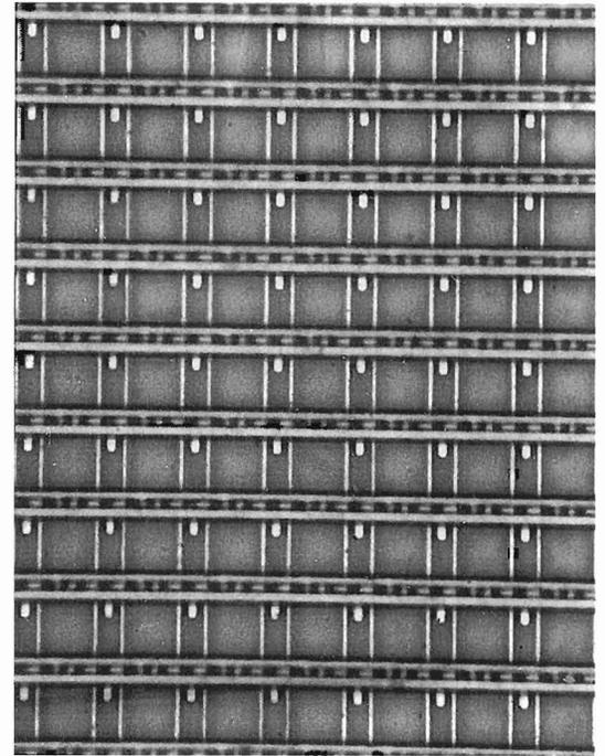
Fig. 4. Close-up of the  $11.9 \mu\text{m}$  pixel photodiode-type active pixels used in the  $1024 \times 1024$  array shown in Fig. 8.
