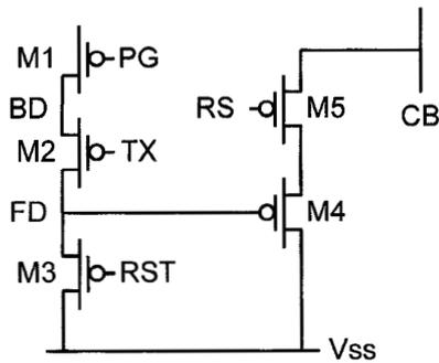
Figure 2: Pixel schematic circuit.
