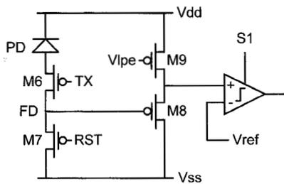
Figure 3: Schematic illustration of event detector circuitry (one of four).
