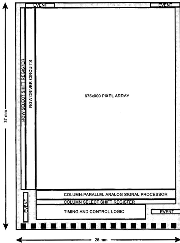
Figure 1: Floorplan of dental CMOS APS.
