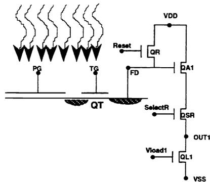
Fig. 3 Single-Polysilicon Active Pixel.
