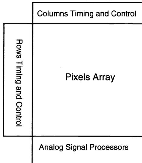
Fig. 1 Architecture of the 256 X 256 CMOS Active Pixel Image Sensor.
