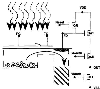
Fig. 2 Double-Polysilicon Active Pixel.
