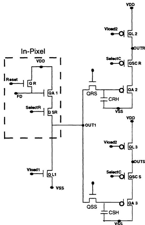
Fig. 4 On-Chip Analog Signal Processor.
