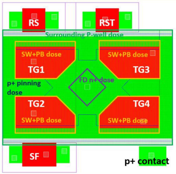
FIGURE 5. 1 \mu\text{m} -pitch, pump-gate jot with four-way shared readout layout, not including deep p-well masks and metal layers. The shape of TGs are optimized to avoid possible potential barrier due to 3-D effects.
