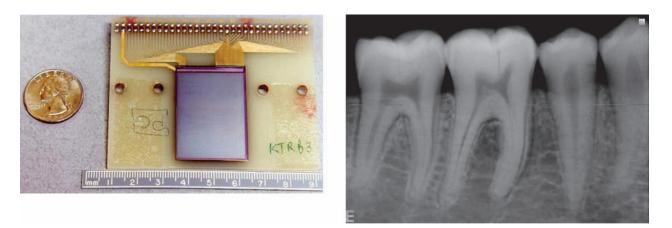
Figure 7. Early CMOS APS sensor for dental X-ray applications and associated X-ray image.
