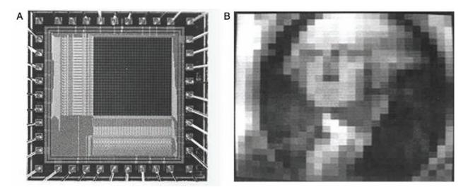
Figure 2. First CMOS APS chip (A) and image captured by chip displayed on a monitor, George Washington from a US \$1 bill (B).
