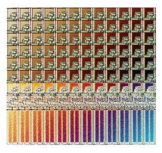
Figure 5. First CMOS APS with pinned photodiode (Kodak and JPL).
