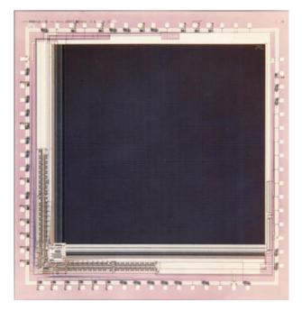
**Figure 3.** JPL CMOS APS camera-on-a-chip with a 256×256 array circa 1994.
