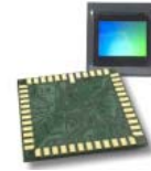
CMOS active-pixel sensor, "camera on-a-chip"
